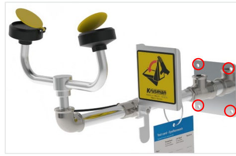
Figure 3: Wall mount for eyewash with four holes pattern 4x Ø8
